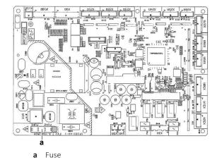
Blown fuse on the Branch selector box PCB?
