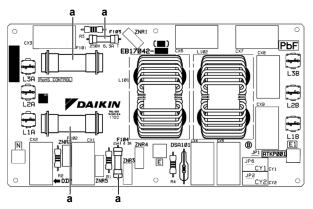
Fuse Blown fuse on the noise filter PCB? Action Replace the noise filter PCB, see Yes "3.12.2 Repair procedures" [▶ 301]. No Return to "3.12.1 Checking procedures" [▶ 298] of the noise filter PCB and continue with the next procedure.
