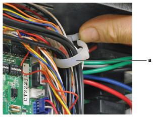
2 Unlatch the cable clamp at the top right corner of the main PCB to facilitate the removal of the PCB.
