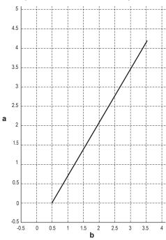
Detected pressure (MPa) Output voltage (V)
